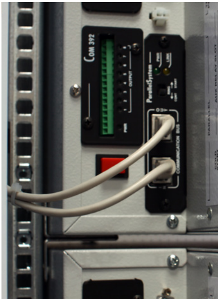
Parallel configuration and programmable relay contacts board
